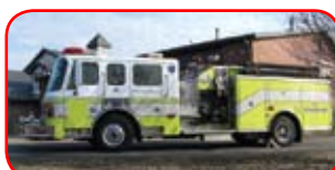
2003 ALF Eagle Rescue Pumper Detroit 430 HP Series 60 Allison HD4060 Automatic Waterous 1500 GPM Pump 500 Gallon Poly Tank
