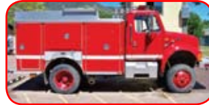
1998 E-One / Int'l 4x4 CAFS Pumper Int'l 210 HP, Allison Automatic Pneumax 120-60 CAF System 400 Gallon Water Tank 20 Gallon Foam Tank Winch on Front Bumper
