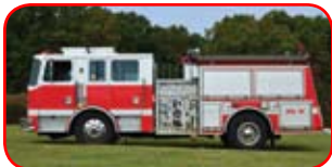
1997 KME Renegade Custom Pumper Detroit Series 60 400 HP Diesel Allison HD4060 Automatic Waterous 1500 GPM Side-Mount Pump 500 Gallon Polypropylene Tank
