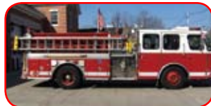
1993 E-One Cyclone Custom Pumper Cummins 300 HP Diesel Engine Allison Automatic Transmission Hale 1500 GPM Side-Mount Pump 750 Gallon Polypropylene Tank
