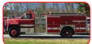
1992 E-One / GMC Pumper Cummins 3116 215 HP Diesel Allison MT643 Automatic Hale QSG 1250 GPM Side-Mount Pump 1000 Gallon Poly Tank
