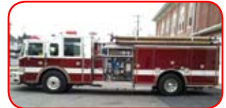
2001 Pierce Dash Rescue Pumper Detroit Series 60, Allison Automatic 2000 GPM Side-Mount Pump 730 Gallon Tank Foam System w/70 Gallon Cell 10KW Hydraulic Generator
