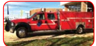
2006 EVI / Ford F-550 Light Rescue International 6.0 Diesel Engine Automatic Transmission 2 - 12 Volt 500 Watt Scene Lights Whelen LED Lightbar Brush Guard with Winch
