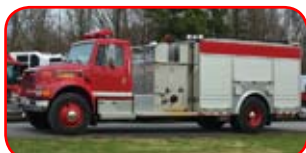
2000 E-One / Int'l Rescue Pumper International 300 HP Diesel Engine Allison MD3060 Automatic Transmission Hale QFLO 1250 GPM Top-Mount Pump 1000 Gallon Poly Tank 2 - 300W Nightfighter Scene Lights
