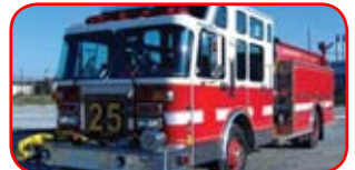
1997 Luerne / Spartan Rescue Pumper Cummins 330 HP, Allison Automatic Hale 1750 GPM Pump Enclosed Pump Panel 1000 Gallon Water Tank AMPS 6KW Hydraulic Generator
