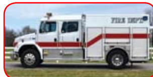
1999 Becker / Freightliner Midi-Pumper Detroit Series 50 320 HP Diesel Allison HD4060 Automatic Waterous CPK-2 300 GPM Pump 300 Gallon Poly Tank
