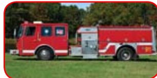
1998 E-One Custom Pumper Diesel, Automatic Hale 1250 GPM Top-Mount Pump 750 Gallon Poly Tank Mileage: 58,000
