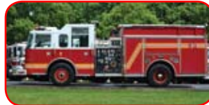
2001 Pierce Saber Rescue Pumper Detroit Series 40 Diesel Engine Allison MD3060 Automatic Waterous CSU 1500 GPM Pump 750 Gallon Poly Tank AMPS 6 KW Hydraulic Generator
