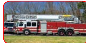
1989 E-One Hurricane 95' Platform Cummins NTC 400 HP, Allison HT740 Hale QSMG 1500 GPM Side-Mount Pump 150 Gallon Aluminum Tank Waterway with Monitor in Platform Onan 6KW Diesel Generator
