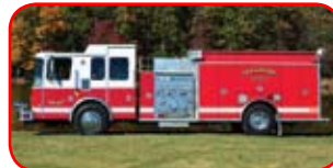
1998 HME Rescue Pumper Detroit Series 40 Diesel Allison WTEC1111 Automatic Hale 1250 GPM Pump w/Enclosed Panel 750 Gallon Poly Tank Onan Generator
