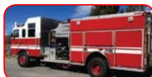
2004 Pierce Dash 4x4 Rescue Pumper Detroit Series 60 515 HP Diesel Allison 4000EVS Automatic Waterous 1500 GPM Top-Mount Pump 500 Gallon Poly Tank Harrison 15 KW Hydraulic Generator
