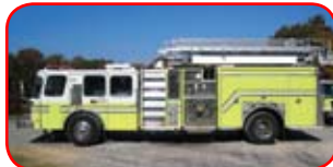
1997 E-One Hurricane 50' Telesboom Detroit Diesel, Allison Automatic Hale 1250 GPM Pump 750 Gallon Poly Tank Combination Monitor at Tip Hydraulic Ladder Rack
