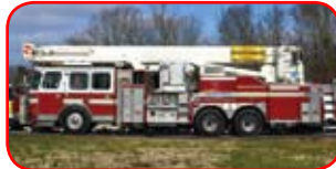
2006 E-One 114' Bronto Platform Bronto Skylift 114' Articulating Aerial Detroit Series 60, Allison EVS4500P Waterous S100 2000 GPM Pump 300 Gallon Poly Tank, Akron Monitor Onan 10KW Hydraulic Generator
