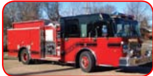
2003 Smeal / Spartan Rescue Pumper Cummins 425 HP, Allison Automatic Waterous 1250 Side-Mount Pump 750 Gallon Poly Tanks Akron Foam System Smart Power 10KW Hydraulic Generator
