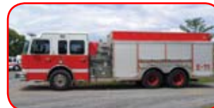
2010 Crimson / Spartan Pumper Tanker Cummins ISL 425 HP, Allison EVS3000 Waterous 1500 GPM Side-Mount Pump 2500 Gallon Poly Tank 3000 Gallon Fold-da-Tank LED Lightbar and DOT Lighting
