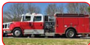
1997 Pierce / FL Rescue Pumper Cummins 300 HP, Allison MD3060 Waterous CS 1250 GPM Side-Mount Pump 500 Gallon Poly Tank 10KW Generator, 3000W Light Tower 12,000# Winch in Front Bumper
