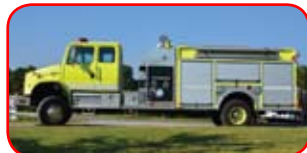
2000 ALF / FL 4x4 Pumper Cummins 350 HP, Allison MD 3066 Hale 1250 GPM Top-Mount Pump 950 Gallon Poly Tank Feecon Foam System
