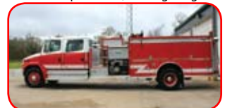
1997 Central States / FL Pumper Cummins 300 HP Diesel Allison MD3060 Automatic Hale 1250 GPM Top-Mount Pump 750 Gallon Poly Tank
