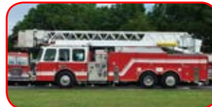
1996 3D / Spartan 100' SkyArm Platform Nova Quintech Articulating Aerial Detroit Series 60, Allison HD4060 Waterous 1500 GPM Pump 300 Gallon Poly Tank AMPS 25KW Generator
