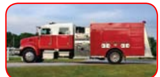
2008 Kenworth Rescue Pumper Paccar PX-8 Diesel, Allison 3000EVS Hale 1500 GPM Side-Mount Pump 500 Gallon Poly Tank Hale Foam Logix Backup Camera, LED Lighting
