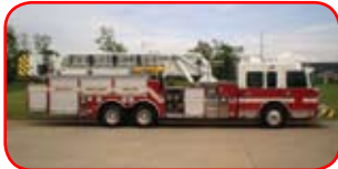
2007 Smeal 100' Mid-Mount Platform Cat C13 525 HP, Allison 4000EVS Waterous S100 1250 GPM Pump 300 Gallon Poly Tank, FoamPro System Onan 10 KW Hydraulic Generator Breathing Air, LED Lighting
