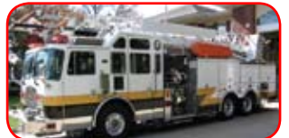
1998 KME Aerial Cat 75' Quint 500 HP Diesel, Allison HD4066 Hale 1500 GPM Pump 500 Gallon Water Tank 9KW PTO-Driven Generator Mileage: 38,392
