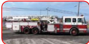
2002 American LaFrance 100' Quint Detroit Series 60 500 HP Engine Allison HD4060P Automatic 2000 GPM Pump 300 Gallon Poly Tank Harrison 10KW Hydraulic Generator
