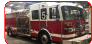
2006 Sutphen Rescue Pumper w/ CAFS Cummins ISM, Allison EVS4000 Hale 1750 GPM Top-Mount Pump 500 Gallon Poly Tank, Hale CAF System Onan 8KW Hydraulic Generator Adjustable Shelves and Slide-Out Trays
