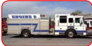
2002 ALF Eagle Rescue Pumper Cummins ISM, Allison HD4060 Waterous 1500 GPM Top-Mount Pump 500 Gallon Tank, 2 - Foam Cells FoamPro A and B Foam System Light Tower, 10KW Generator
