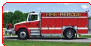
1994 Southern Coach / FL Pumper Cummins Diesel, Allison MT643 Darley 1000 GPM Front-Mount Pump 750 Gallon Poly Tank Gas Generator, LED Lightbar
