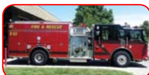
2003 Pierce Dash Rescue Pumper Detroit 475 HP, Allison 4000EVS Hale QMAX 1250 GPM Side-Mount Pump 500 Gallon Poly Tank Smart Power 8KW Generator 1 - Electric Cord Reel
