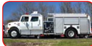
2000 Pierce / Int'l Rescue Pumper Int'l 530E 300HP, Allison MD3060 Waterous 1000 GPM Side-Mount Pump 500 Gallon Poly Tank AMPS 8KW Hydraulic Generator Will-Burt 25' 4000W Light Tower
