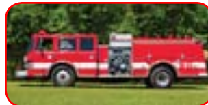
1992 Pierce Arrow Rescue Pumper Detroit Diesel, Allison MT Waterous CMU 1750 GPM Pump 750 Gallon Steel Tank Onan 3 KW Diesel Generator
