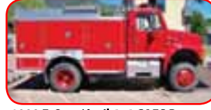
1998 E-One / Int'l 4x4 CAFS Pumper Int'l 210 HP, Allison Automatic Pneumax 120-60 CAF System 400 Gallon Water Tank 20 Gallon Foam Tank Winch on Front Bumper
