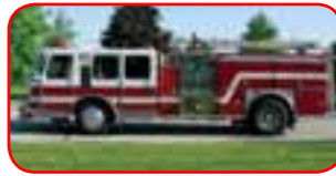
1989 E-One Hurricane Rescue Pumper Cummins NTC 400 HP Diesel Allison HT4060 Automatic Hale 1250 GPM Side-Mount Pump 500 Gallon Poly Tank 8000# Winch on Front Bumper
