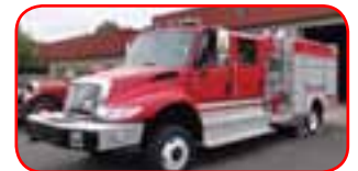
2008 Crimson / Int'l 4x4 Interface Pumper Navistar 300 HP, Allison 2500EVS Waterous CXV 1000 GPM Pump 500 Gallon Poly Tank Hale HPX300-B18 Auxiliary Pump FoamPro 1600 System
