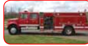
2001 Sutphen / Int'l Rescue Pumper International CL 300 HP Diesel Allison MD3060 Automatic Hale 1250 GPM Side-Mount Pump 500 Gallon Fiberglass Tank Onan 4KW Gas Generator
