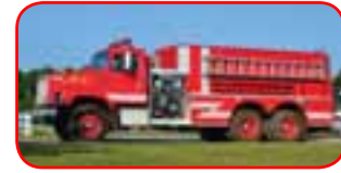
1996 International Pumper Tanker Cummins 300 HP Diesel Engine Waterous 1000 GPM Side Mount Pump 2500 Gallon Poly Tank
