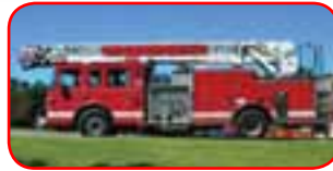
2004 Pierce Dash 75' Quint Caterpillar 455 HP Diesel Engine Allison EVS 4000P Automatic Hale QMAX 1500 GPM Pump 450 Gallon Poly Tank
