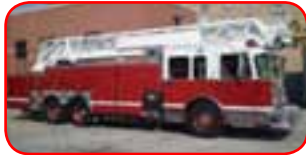
2001 Ferrara / Spartan 105' Aerial Diesel Engine, Automatic Transmission Hydraulic Generator Hydraulic Reel in Bumper
