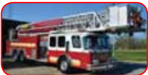
1996 E-One Hurricane 105' Platform Detroit 8V92 500 HP Diesel Engine Allison HD4060 Automatic Transmission Hale QSMG 1500 GPM Pump 150 Gallon Poly Tank 6KW Hydraulic Generator
