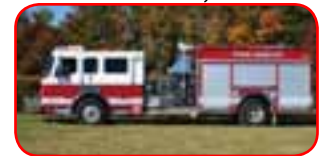
2004 American LaFrance Rescue Pumper Cummins 330 HP Diesel Engine Automatic Transmission 1250 GPM Side-Mount Pump 1000 Gallon Poly Tank Foam Pro 2001 A&B Foam System
