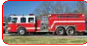
1996 E-One Custom Pumper Tanker Detroit 8V92 370 HP Diesel Allison HT740D Automatic Hale 1500 GPM Side-Mount Pump 1900 Gallon Poly Tank
