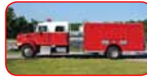
2008 Kenworth Rescue Pumper Paccar PX-8 Diesel, Allison 3000EVS Hale 1500 GPM Side-Mount Pump 500 Gallon Poly Tank Hale Foam Logix Backup Camera, LED Lighting
