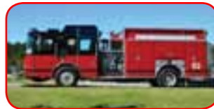
2007 Ferrara Intruder Rescue Pumper Cummins ISC 330 HP, Allison 3000EVS Waterous CSM 1500 GPM Pump 1000 Gallon Poly Tank Seating for 6 - 5 SCBA Seats Booster Reel, Slide-out Rear Tray
