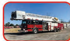
2001 Seagrave 105' Tower Waterous 2000 GPM Pump 300 Gallon Tank Detroit Diesel
