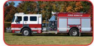
2004 American LaFrance Rescue Pumper Cummins 330 HP Diesel Engine Automatic Transmission 1250 GPM Side-Mount Pump 1000 Gallon Poly Tank Foam Pro 2001 A&B Foam System
