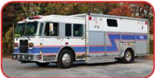
2004 Spartan Walk-In Heavy Rescue Cummins ISC 330 HP, Allison EVS3000 Onan 10KW PTO-Driven Generator 6-Bottle 6000psi Cascade System Hitch Receivers on Front and Rear Awning on Driver's Side
