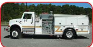
1999 KME / International 4x4 Pumper International 250 HP Diesel Engine Allison Automatic Transmission Hale 1250 GPM Side-Mount Pump 500 Gallon Polypropylene Tank 3300 Watt Hydraulic Generator
