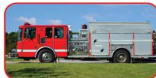
2000 Central States Rescue Pumper Cummins ISM, Allison MD3066 Hale DSD 1500 Side-Mount Pump 750 Gallon Poly Tank Class B ATP Foam System FoamPro 1600 Class A Foam System
