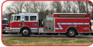
1997 KME Custom Rescue Pumper Detroit 325 HP, Allison MD3060P Hale QSMG 1500 GPM Top-Mount Pump 900 Gallon Poly Tank, Foam System 2 - 10 Gallon Foam Cells Aluminum Hose Bed Cover
