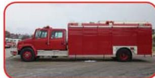
1994 Freightliner Heavy Rescue Cummins 8.3L 300 HP Diesel Engine Allison Automatic Transmission Winco 20KW PTO Generator Wilbur Light Tower
