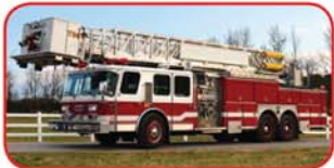
1990 E-One Hurricane 95' Platform Detroit 8V92, Allison HT 740 Hale QSMG 1500 GPM Pump 200 Gallon Polypropylene Tank Onan 6000 Watt Diesel Generator Mileage: 12,945
