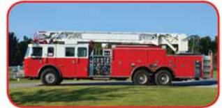
2002 Pierce Lance 75' Quint Cummins ISM 500 HP, Allison HD 4060P Waterous CMU 2000 GPM Pump 500 Gallon Poly Tank 8KW Hydraulic Generator Automatic Tire Chains
