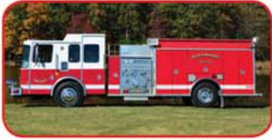
1998 HME Rescue Pumper Detroit Series 40 Diesel Allison WTEC1111 Automatic Hale 1250 GPM Pump w/Enclosed Panel 750 Gallon Poly Tank Onan Generator
