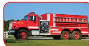
1996 International Pumper Tanker Cummins 300 HP Diesel Engine Waterous 1000 GPM Side Mount Pump 2500 Gallon Poly Tank
