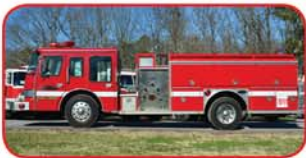
1988 E-One Hush Custom Pumper Detroit 6V92 Rear-Mount Diesel Allison HT 740 Automatic Hale QSMG 1500 GPM Top-Mount Pump 500 Gallon Aluminum Tank
