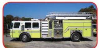
1997 E-One Hurricane 50' Teleboom Detroit Diesel, Allison Automatic Hale 1250 GPM Pump 750 Gallon Poly Tank Combination Monitor at Tip Hydraulic Ladder Rack
