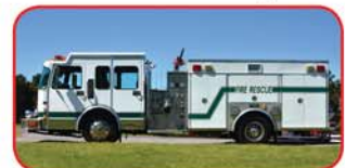
1998 Saulsbury / Spartan Rescue Pumper Detroit Series 60 470 HP Diesel Allison HD4060 Automatic Waterous 2000 GPM Side-Mount Pump 800 Gallon Poly Tank
