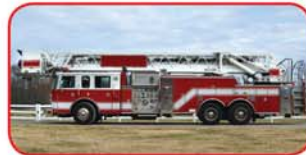
2000 Pierce Dash 100' Platform Detroit Series 60, Allison 4060PR Waterous 1500 GPM 2-Stage Pump 300 Gallon Poly Tank 2 - 1500 GPM Monitors 10KW Hydraulic PTO Generator
