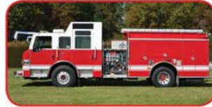
2007 Pierce Velocity Rescue Pumper Detroit Series 60, Allison 4000EVS Waterous 1500 GPM Side-Mount Pump 750 Gallon Poly Tank Huskey Foam System with CAFS LED Lighting Package
