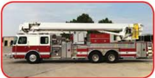
2002 E-One 118' Bronto Platform Bronto Skylift Articulating Aerial Diesel Engine, Allison Automatic Hale QMAX 2000 GPM Pump 200 Gallon Poly Tank Breathing Air to Tip
