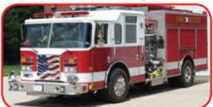
2003 Pierce Dash Rescue Pumper Detroit 500 HP, Allison Automatic Waterous 1250 GPM Pump, Hercules CAFS 1000 Gallon Poly Tank, 2 - Foam Cells Harrison 5KW PTO Generator Command Light Tower
