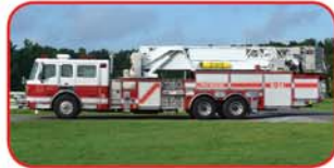
2004 American LaFrance 93' Platform Detroit 500 HP, Allison 4000EVS Hale 1500 GPM Pump 200 Gallon Poly Tank Harrison Hydraulic Generator Breathing Air to Platform
