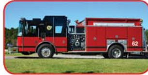
2007 Ferrara Intruder Rescue Pumper Cummins ISC 330 HP, Allison 3000EVS Waterous CSM 1500 GPM Pump 1000 Gallon Poly Tank Seating for 6 - 5 SCBA Seats Booster Reel, Slide-out Rear Tray
