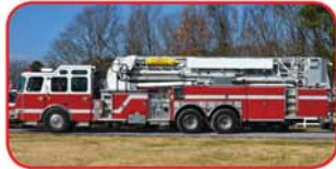
2007 E-One 95' Mid-Mount Platform Cummins 500 HP, Allison Automatic Hale 8GFR 2000 GPM Pump 250 Gallon Poly Tank Monitor in Platform
