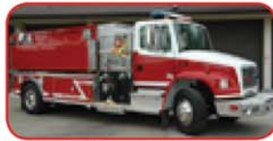
2001 Central States / FL Pumper Tanker Cummins ISC 330 HP Diesel Engine Allison Automatic Transmission 750 GPM Side-Mount Pump 1800 Gallon Booster Tank 3 - Dump Valves, LS, RS, and Rear
