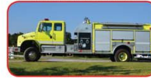
2000 ALF / FL 4x4 Pumper Cummins 350 HP, Allison MD 3066 Hale 1250 GPM Top-Mount Pump 950 Gallon Poly Tank Feecon Foam System
