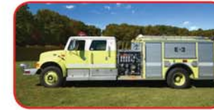
2002 Pierce / Int'l Rescue Pumper Int'l 330 HP Diesel, Allison MD3060 Waterous 1250 GPM Side-Mount Pump 500 Gallon Polypropylene Tank FoamPro System with 2 - 10 Gallon Cells AMPS PTO Diesel Generator
