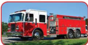
1999 Ferrara / Spartan Pumper Tanker Cummins 330 HP Diesel Hale QSG 1250 GPM Top-Mount Pump 2000 Gallon Poly Tank Dump Valve in Rear Mileage: 30,606
