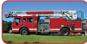
2004 Pierce Dash 75' Quint Caterpillar 455 HP Diesel Engine Allison EVS 4000P Automatic Hale QMAX 1500 GPM Pump 450 Gallon Poly Tank
