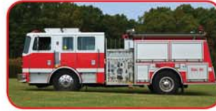
1997 KME Renegade Custom Pumper Detroit Series 60 400 HP Diesel Allison HD4060 Automatic Waterous 1500 GPM Side-Mount Pump 500 Gallon Polypropylene Tank
