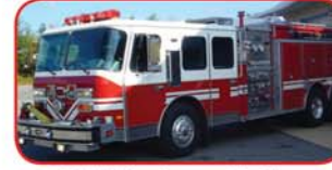
1991 E-One Pumper Tanker Detroit 8v92, Allison HT740 Have QSMG 1500 GPM Pump 2000 Gallon Water Tank Feecon Foam System Onan 7.5KW Generator
