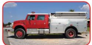
1999 3D / Int'l 4x4 Interface Pumper Int'l DT466 Diesel Engine Allison MT643 Automatic Darley HE 500 GPM Auxiliary Pump 250 HP Diesel Pump Engine 750 Gallon Poly Tank
