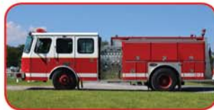
1994 E-One Sentry Custom Pumper Cummins 300 HP, Allison MD3060 Hale 1250 GPM Side-Mount Pump 750 Gallon Poly Tank Automatic Tire Chains
