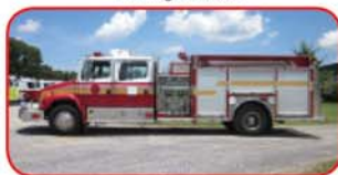
2000 ALF / Freightliner Pumper Cummins 300 HP Diesel Allison MD3060 Automatic Hale 1250 GPM Side-Mount Pump 750 Gallon Poly Tank
