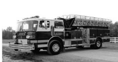
$65,000 1984 Sutphen 65' Mini Tower 1500 Hale Pump 500 Gallon Tank Detroit 8V-71 Diesel Allison Automatic
