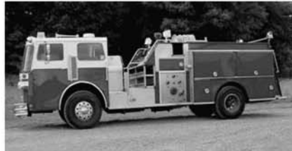
$39,000 1985 Sutphen Pumper 1500 Hale Top-Mount 750 Gallon Fiberglass Tank Detroit 8V-92TA Diesel Allison Automatic
