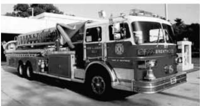
$80,000 1981 Sutphen 100' Tower 1500 Hale Pump 300 Gallon Tank Detroit 8V-71 Diesel Allison Automatic
