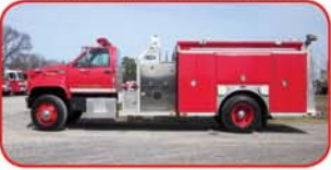
2001 E-One / GMC Commercial Pumper Cat 3126 246HP Diesel Allison MD3060 Automatic Hale 1250 GPM Top-Mount Pump 1000 Gallon Poly Tank
