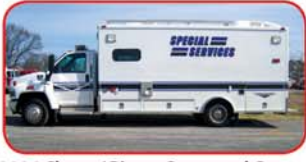
2006 Chevy / Pierce Command Center Duramax Diesel, Allison Automatic 10KW Diesel Generator 1/3" CCD Telescoping Camera Sink, Refrigerator, Microwave 2 - 20" Flat Panel Televisions
