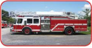
1993 E-One Hurricane 75' Quint Cummins 350 HP Diesel Allison HT740 Automatic Hale QSMG150-23 1500 GPM Pump 500 Gallon Poly Tank
