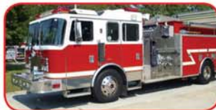
1996 KME Renegade Rescue Pumper Caterpillar 6CTA 300 HP Diesel Allison MD3060P Automatic Hale 1500 GPM Top-Mount Pump 1000 Gallon Poly Tank
