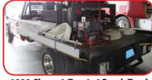
1999 Chevy 1-Ton 4x4 Brush Truck Gas Engine, Automatic Transmission 200 GPM Gas-Powered Pump 250 Gallon Tank 5KW Generator
