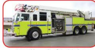
2001 Pierce Dash 75' Quint Detroit Diesel, Allison Automatic Hale QMAX 2250 GPM Pump FoamPro 1600 Class A System 480 Gallon Poly Tank AMPS 15 KW Hydraulic Generator
