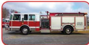
1997 Southern Coach Pumper Cummins C8.3 325 HP Diesel Engine Allison MD 3060 Automatic Transmission Hale 1500 GPM Side-Mount Pump 750 Gallon Poly Tank
