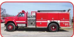
1998 Ford/E-One Pumper Cummins 8.3L 250 HP Diesel Engine Allison Automatic Transmission Hale 1250 GPM Side-Mount Pump 1000 Gallon Poly Tank Piped for Deck Gun
