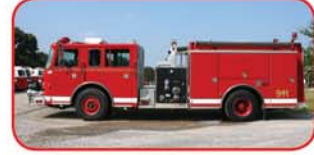
1998 Pierce Saber Custom Pumper Cummins 8.3L 325 HP Diesel Allison MD3060 Automatic 1250 GPM Waterous Top-Mount Pump 1000 Gallon Poly Tank
