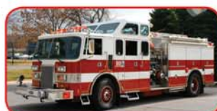
1989 Pierce Lance Rescue Pumper Cummins 350 Horsepower Diesel Allison Automatic Transmission Waterous 1500 GPM Side-Mount Pump 1000 Gallon Steel Tank
