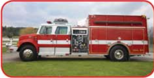
1999 Pierce / Int'l Pumper / Tanker International 320 HP Diesel Allison MD3060 Automatic Waterous 1250 GPM Side-Mount Pump 1500 Gallon Poly Tank Honda 5KW Generator
