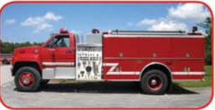
2000 KME/Chevy Commercial Pumper Caterpillar 3126 246 HP Diesel Engine Allison MD3060 Automatic Transmission Hale 1250 GPM Side-Mount Pump 1000 Gallon Poly Tank Akron/Apollo Deck Gun
