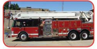
1986 Pierce Lance 100' Quint Detroit 8V92 Diesel Engine Allison Automatic Waterous 1250 GPM 2-Stage Pump Onan 12KW Diesel Generator
