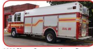
1998 Pierce Quantum Heavy Rescue Detroit Diesel, Allison Automatic Hale AP 500 GPM Pump 250 Gallon Poly Tank Winco 25KW PTO Generator Nightscan Light Tower
