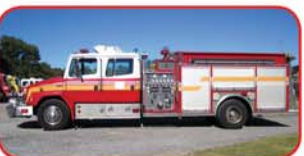
1998 SC/FL Rescue Pumper Cummins 300 HP Diesel Allison MD3060 Automatic Hale QSMG 1250 GPM Pump 750 Gallon Poly Tank
