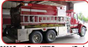
2006 Foust Bros / KW Pumper / Tanker Cummins Diesel Allison Automatic Darley 1250 GPM Side-Mount Pump 3000 Gallon Poly Tank 3000 Gallon Drop Tank
