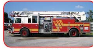
1996 Pierce Lance 75' Quint Detroit 8V92TA 500 HP Diesel Allison HD4060PR Automatic Hale QSMG150 1500 GPM Pump 300 Gallon Poly Tank Onan 6KW Diesel Generator
