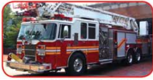
1998 Pierce Dash 105' Quint Detroit Series 60 470 HP Diesel Allison HD4060P Automatic Hale QSMG 2000 GPM Pump 300 Gallon Poly Tank FOUR UNITS AVAILABLE
