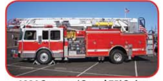
1994 Spartan / Smeal 75' Quint Detroit Series 60 450 HP Diesel Allison HT740 Automatic Waterous 1500 GPM 2-Stage Pump 300 Gallon Poly Tank Akron 95 GPM Foam System
