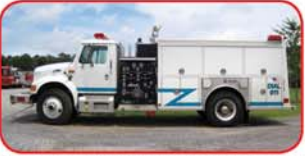
2000 Summit / International Pumper Diesel Engine, Automatic Transmission 1250 GPM Pump 1000 Gallon Poly Tank 10" Newton Dump in Rear
