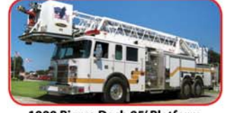
1999 Pierce Dash 85' Platform etroit Series 60 500 HP Diesel Allison HD-4060PR Automatic Waterous CMU YCK 1500 GPM Pump 300 Gallon Poly Tank FoamPro System w/ 20 Gallon Tank
