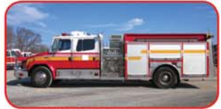
2001 ALF / Freightliner Rescue Pumper Cummins 300 HP Diesel Allison MD3060 Automatic Hale QSMG 1250 GPM Pump 750 Gallon Poly Tank
