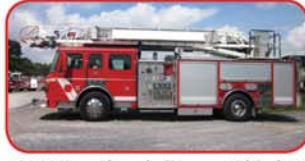
2002 American LaFrance 75' Quint Cummins ISM 400HP Diesel Allison MD3060P Automatic Hale 1250 GPM Side-Mount Pump 400 Gallon Poly Tank 6KW Hydraulic PTO-Driven Generator
