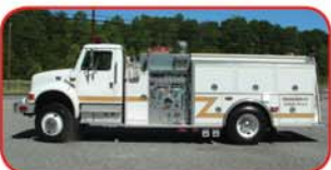
1999 KME / International 4x4 Pumper International 250 HP Diesel Allison Automatic Transmission Hale 1250 GPM Side-Mount Pump 500 Gallon Poly Tank 3300 Watt Diesel Generator
