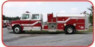
1998 Ford/E-One Pumper Cummins 8.3L 250 HP Diesel Engine Allison Automatic Transmission Hale 1250 GPM Side-Mount Pump 1000 Gallon Poly Tank Piped for Deck Gun
