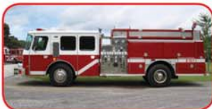
1990 E-One Cyclone Custom Pumper Cummins 404 Diesel Allison HT740 Automatic Hale QSMG 1500 GPM Side-Mount Pump 750 Gallon Poly Tank 30 Gallon Foam Tank
