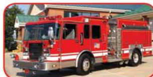
1995 Spartan / Saulsbury Pumper Diesel Engine Automatic Transmission 1250 GPM Side-Mount Pump 1000 Gallon Poly Tank
