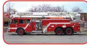
1993 Pierce Arrow 105' Quint Detroit 8V92TA 450 HP Diesel Allison HT740 Automatic Waterous 1500 GPM Pump 500 Gallon Tank Onan Generator
