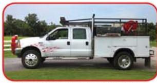
2001 Ford F-550 4x4 Brush Truck Ford 7.3L Powerstroke Diesel Ford 2711F Manual 100 GPM Pump 300 Gallon Polypropylene Tank Foam-It System with 20 Gallon Tank
