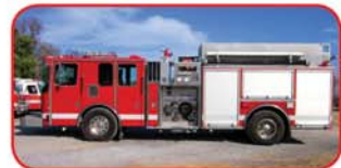
1993 HME/Quality Pumper Detroit 6V92 400 HP Diesel Engine Automatic Transmission Waterous 1750 GPM Pump 500 Gallon Poly Tank Onan 12KW Diesel Generator
