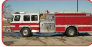
1999 E-One Cyclone Rescue Pumper Cummins ISM 320 HP Diesel Allison MD3060 Automatic Hale 1250 GPM Side-Mount Pump 500 Gallon Poly Tank
