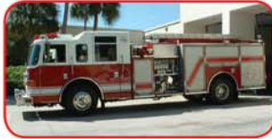
2002 Pierce Enforcer Rescue Pumper Cummins ISL 370 HP Diesel Allison MD3066 Automatic Waterous 1250 GPM Side-Mount Pump 500 Gallon Poly Tank
