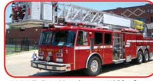
1994 E-One Hurricane 95' Platform Detroit 8V92 450 HP Diesel Allison HT740 Automatic Waterous 2000 GPM Pump 200 Gallon Poly Tank Foam System
