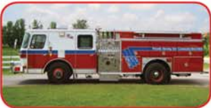
1990 E-One Hush Rescue Pumper Detroit 6V92 Diesel Engine Allison HT741 Automatic Hale 1500 GPM Side-Mount Pump 500 Gallon Polypropylene Tank Akron Foam System w/20 Gallon Tank
