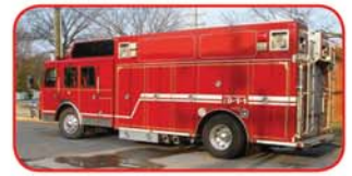
1994 E-One Protector Heavy Rescue Cummins 8.3L Diesel Engine Allison 3060 Automatic 25kW PTO-Driven Generator Will-burt Light Tower 12,000# Winch in Front Bumper
