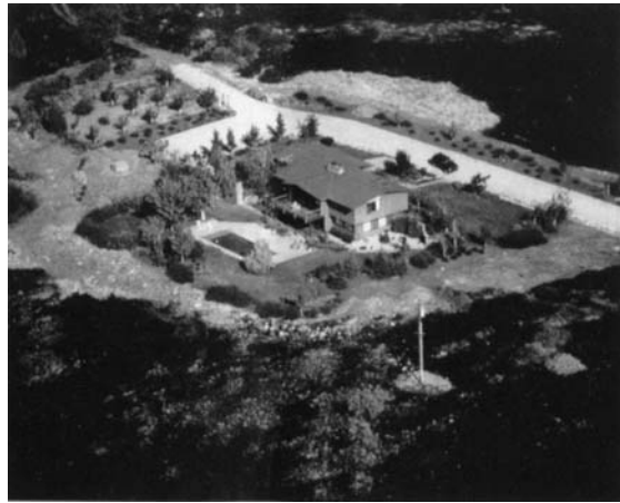
The pre-fire activities implemented by this homeowner included a green and well maintained landscape, reduction of wild vegetation around the perimeter of the property, a fire-resistant roof, and a good access road with a turnaround area. As seen in the photo, these pre-fire activities were effective.
