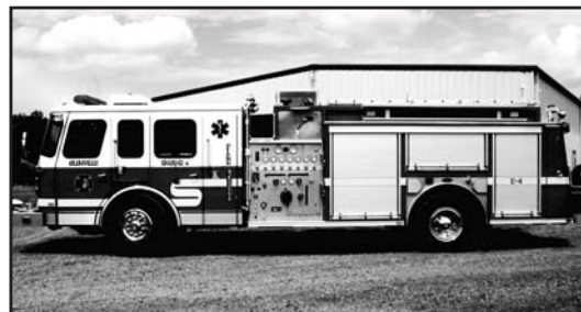
1995 E-One Rescue Pumper 1250 Hale Pump 500 Gallon Poly Tank Hydraulic/Electric Reel $110,000
