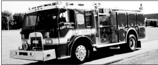
1985 Kenworth/FMC Pumper 5 Man Cab Diesel/Automatic 1000 GPM Pump/1000 Poly Tank
