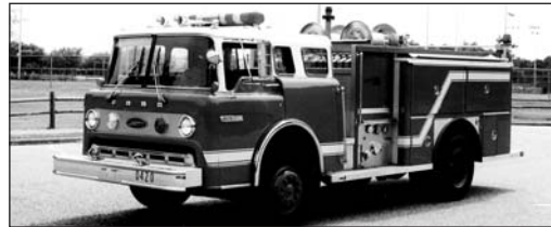
1980 Ford E-One 5 Man Cab Diesel/Automatic 1000 GPM Top Pump/750 Gallon Tank
