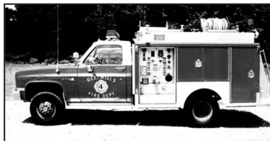
1981 Mini-Pumper 250 GPM Hale PTO Pump 250 Gallon Pump Gas/4-Speed $13,000
