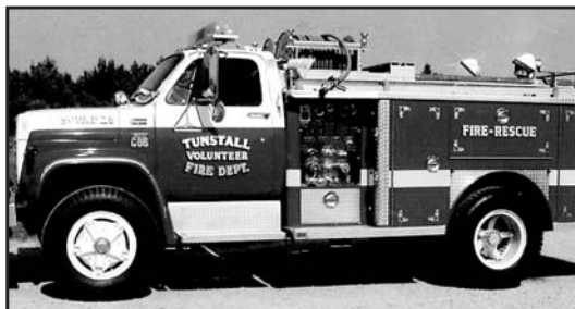
1978 E-One Mini-Pumper 250 GPM PTO Pump 300 Gallon Tank Gas V-8/Automatic $15,000
