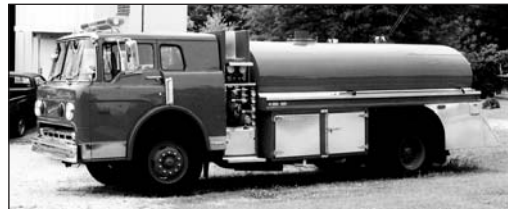
1985 TANKER Diesel Automatic 400 GPM Pump 2000 Gallon Stainless Steel Tank
